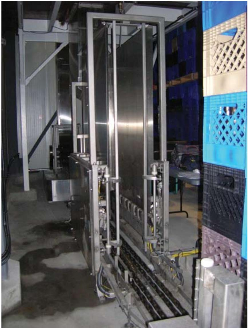
*Bottom-Out Destacking operates at up to 90 cases/minute.*
