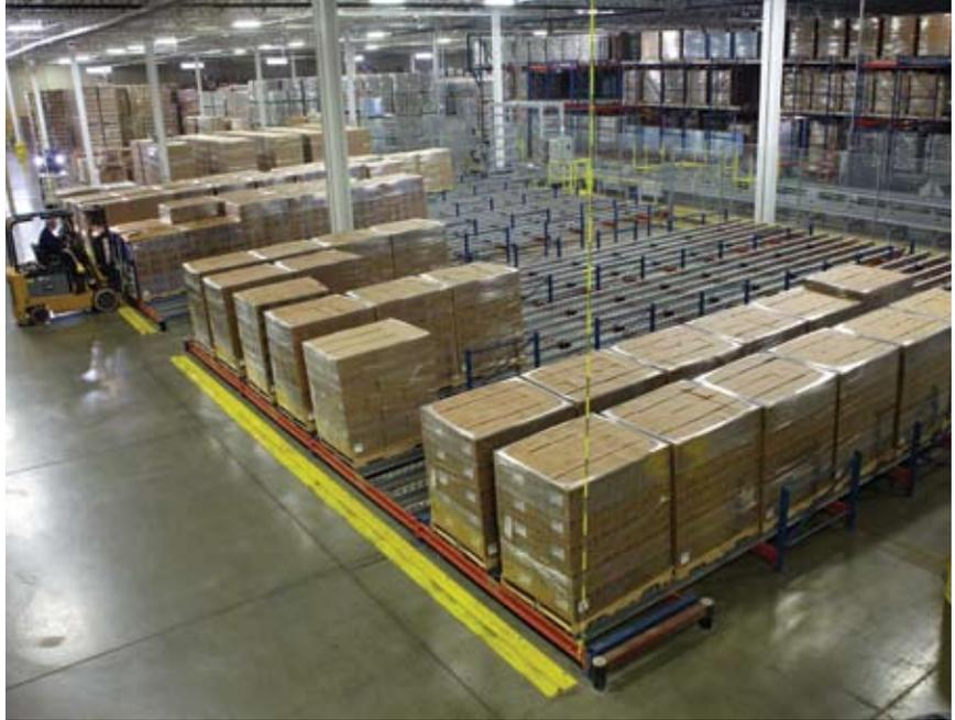
fer peak shipping and receiving volumes. The multi-aisle AS/RS design is based on Westfalia's multiple deep Satellite® technology, which provides the ability to create a compact, 6- to 11-pallet deep storage solution. Storing pallets 3 levels in the 22' high facility maximizes storage density, thereby negating the need for a new building and possible construction costs. Included in the AS/RS are conveyors, 6 Storage Retrieval Machines (SRMs) with Satellite® rack entry vehicles, and WMS
