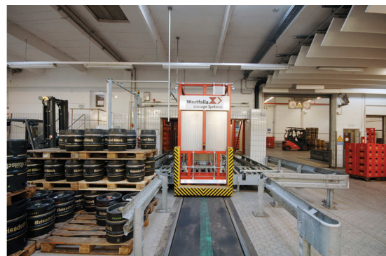
Figure 3. Transfer car with inductive power supply at the disposal station in the bottling and barreling production areas.
