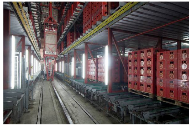
Figure 4. Rack aisle for one of two storage/retrieval machines at the Reissdorf warehouse.
