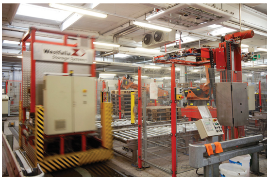
Figure 3. Transfer car with inductive power supply at the disposal station in the bottling and barreling production areas.
