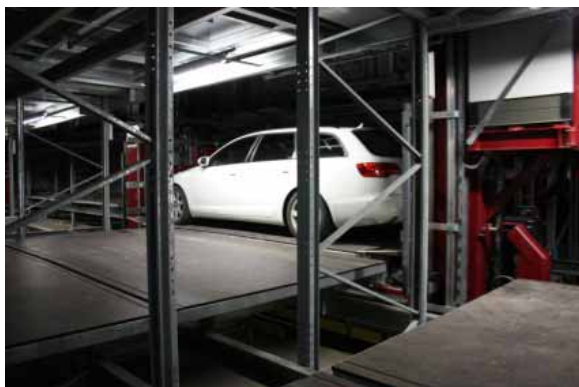
Photo: Insight into the depths - the Storage Retrieval Machine (SRM) carries the car to the scheduled location.
