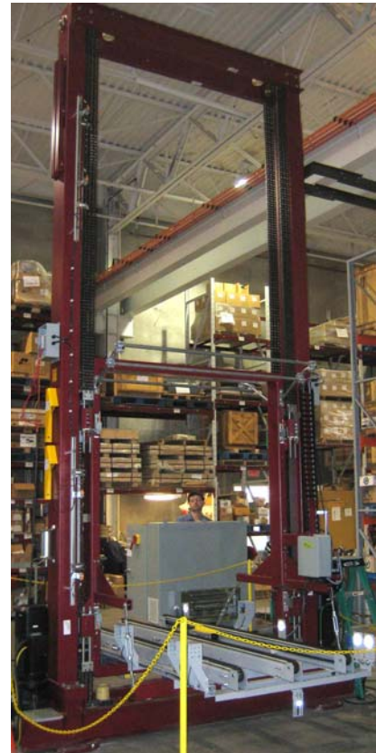
Vertical Lift under construction
