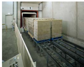
Picture 3: Automated conveyor with turn table at a Kloosterboer cold store near Rotterdam
